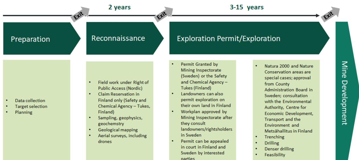
**Fig. 3. The different phases of mineral exploration and the formal permitting processes in Finland and Sweden.**
