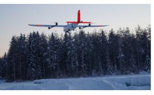
Drone equipped with electromagnetic survey system for mineral exploration
